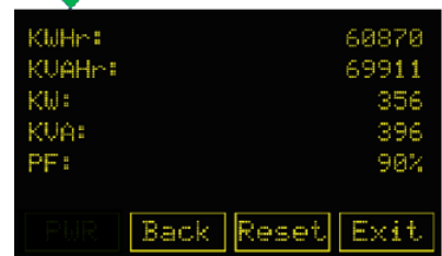
Power Metering Screen
