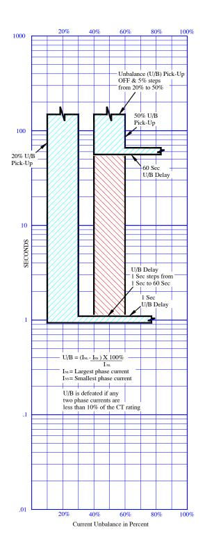
Figure 18.5: Phase Current Unbalance TCC
