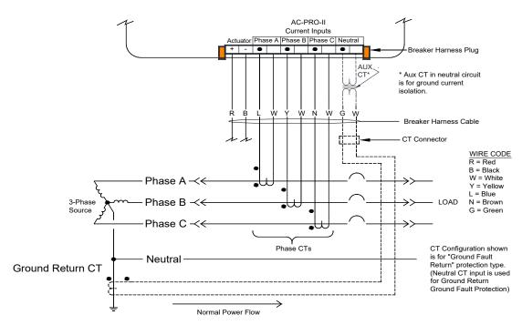
Figure 5.4: AC-PRO-II Typical Ground Return Wiring Diagram
