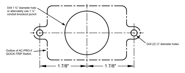
Figure 7.3: AC-PRO-II QT2-Switch Drilling Plan (Verify Printer Scaling prior to Drilling)
