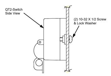
Figure 7.4: QT2-Switch Mounting
