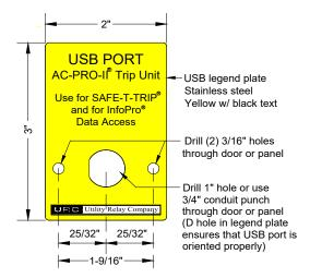
Figure 5.7: USB Extension Plate Drilling
