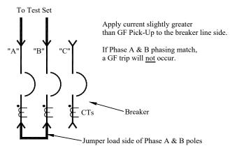
Figure 14.2: Phase A & B, CT Polarity Test
