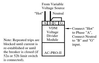
Figure 14.6: Overvoltage Test (temporary connections)
