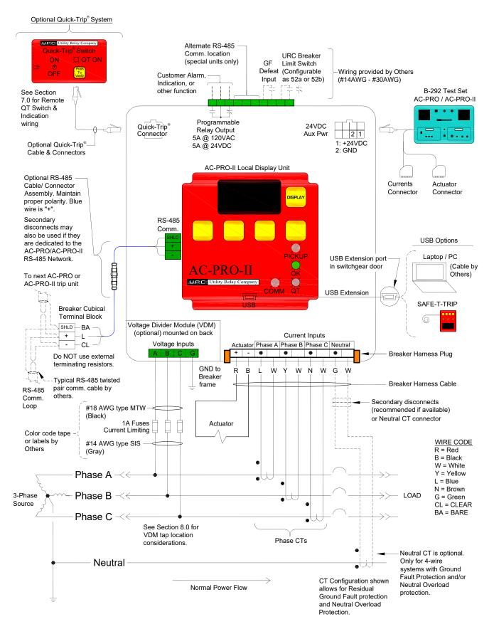
Figure 5.3: AC-PRO-II Typical Wiring Diagram
