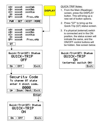
Figure 7.8: Front Panel QUICK-TRIP ON/OFF Control
