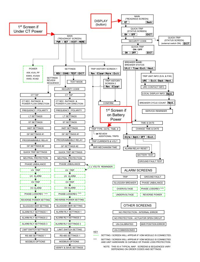
Figure 6.3: Typical AC-PRO-II Menu Navigation Map - Simple View
