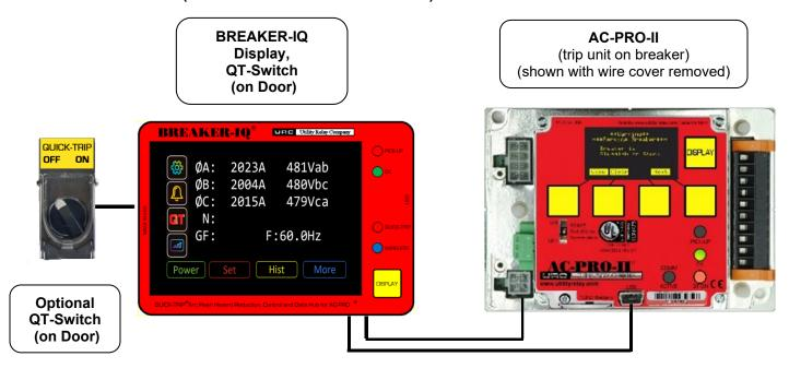
Figure 7.1: QUICK-TRIP System and Connections (Option #1, includes BREAKER-IQ display)
