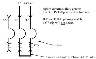
Figure 14.3: Phase B & C, CT Polarity Test
