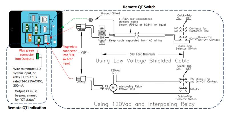
Figure 7.6: BREAKER-IQ Display with Remote QT Switch & Indication
