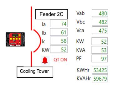
Figure 24.4: Smart 1-Line / Breaker Status and Alarms Screen
