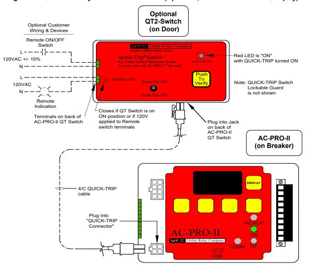
Figure 7.2: QT2-Switch Connections (Option #2, no display)
