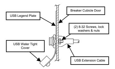
Figure 5.8: USB Extension Plate & Cable Installation
