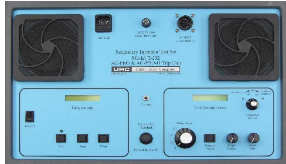
Figure 15.1: B-292 Secondary Injection Test Set
